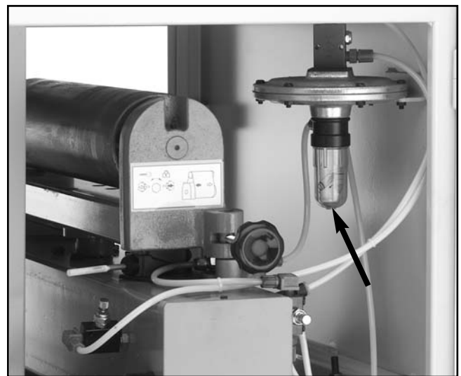
Figure 19. Unscrew this filter to empty it.
